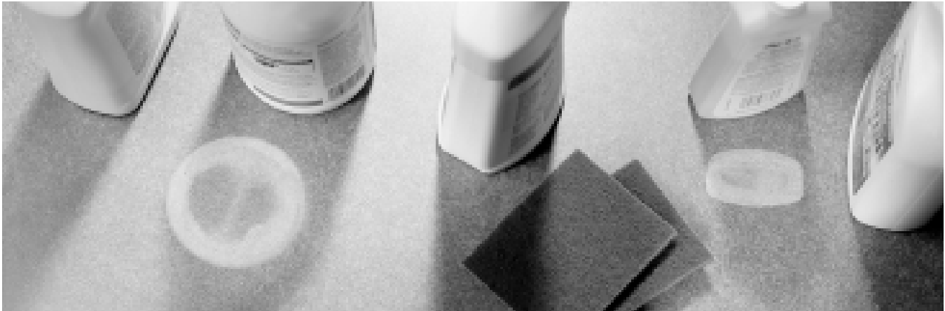
Typical damage that can occur to laminate when exposed to harsh chemicals.
